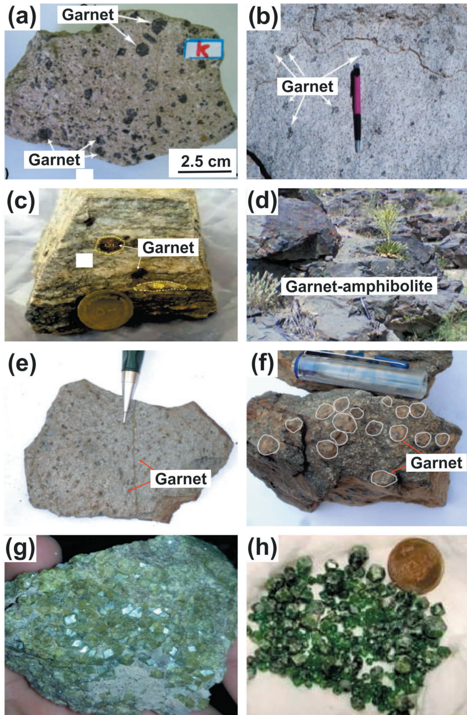
Figure 7. Representative photos of garnetiferous granitoids, metamorphic rocks, and ophiolites from south and western Iran. (a, b) Ti-rich andradite garnet in Kaleybar granitoid from the Azerbaijan district (Ashrafi et al., 2009). (c) Almandine garnet in Gol Gohar granite from Kerman district (Safarzadeh et al., 2016). (d) Garnet (almandine-spessartine) in Qarehaghaj amphibolite from the Azerbaijan district (Advay et al., 2017). (e, f) Almandine garnet porphyroblasts in Ruchun and Gol Gohar schists from Kerman district (Fatehi and Ahmadipour, 2017). (g, h) Garnets with andradite-grossular and uvarovite in related to ophiolitic complex from the Soghan region in the Kerman district (Montaseri et al., 2013).
