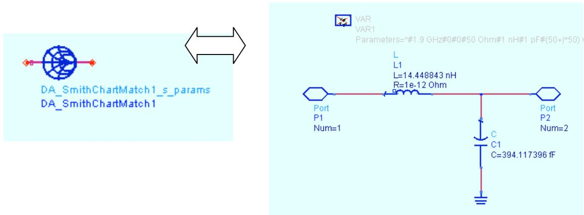
Now it is time to use the matching network with the amplifier. You could use the component by connecting it to the amplifier input. However, because you will be using the optimizer, it is better to have the L-C components on the schematic.
