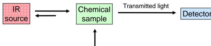
From all the frequencies it receives, the chemical sample can **absorb** (retain) **specific frequencies** and allow the rest to pass through it (transmitted light).
