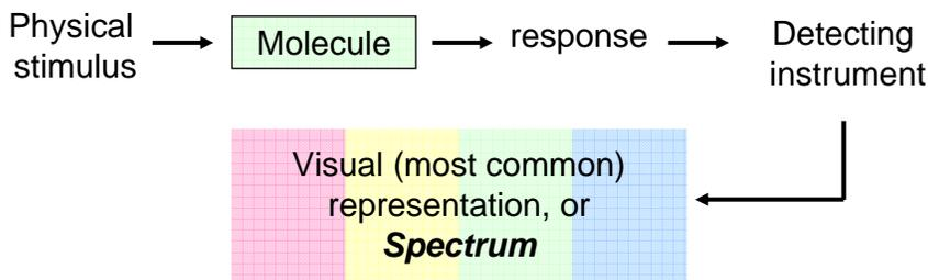
Upon irradiation with infrared light, certain bonds respond by vibrating faster. This response can be detected and translated into a visual representation called a spectrum.
