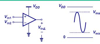
$$V_{out} = \frac{V_{\text{max}} - V_{\text{min}}}{2} \sin \omega t + \frac{V_{\text{max}} + V_{\text{min}}}{2} \quad \omega_{FP} = \frac{SR}{V_{\text{max}} - V_{\text{min}}}$$
