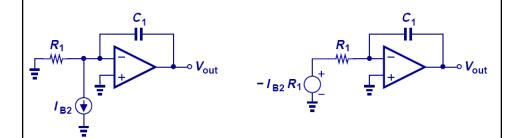
$$V_{out} = -\frac{1}{R_1 C_1} \int (-I_{B2} R_1) dt$$
