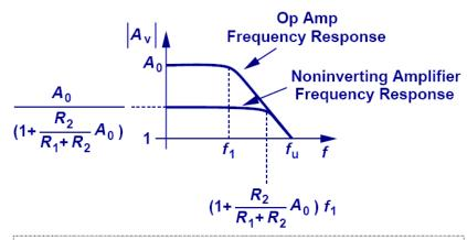
Having a loop around the op amp (inverting, noninverting, etc) helps to increase its bandwidth. However, it also decreases the low frequency gain.
