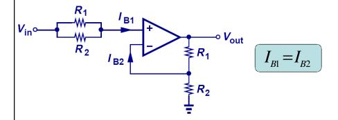
Since the correction voltage is dependent upon β, and β varies with process, we insert a parallel resistor combination in series with the positive input. As long as I<sub>B1</sub>= I<sub>B2</sub>, the correction voltage can track the β variation.
