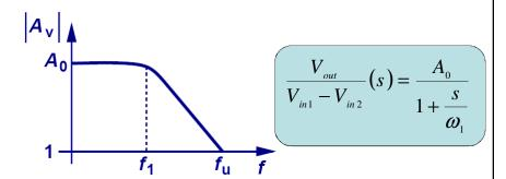
Due to internal capacitances, the gain of op amps begins to roll off.
