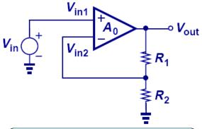
$$\left(\begin{array}{c} \frac{V_{out}}{V_{in}} \approx \left(1 + \frac{R_1}{R_2}\right) \left[1 - \left(1 + \frac{R_1}{R_2}\right) \frac{1}{A_0}\right] \end{array}\right)$$
