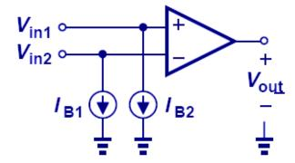
The effect of bipolar base currents can be modeled as current sources tied from the input to ground.
