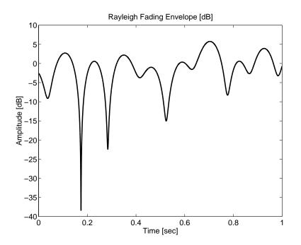
• Using the simulated data for  $f_m = 5$  Hz, LCR= 9 and AFD= 0.0055 when the rms threshold is set to be -10 dB. Based on LCR and AFD equations, we find
