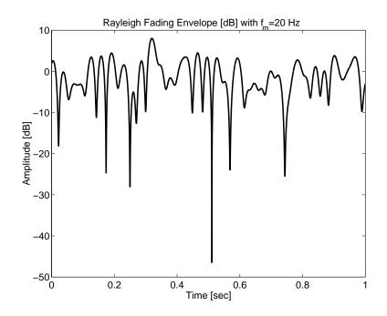
Since the simulated data is relatively short, the simulated results can be somewhat different from the theoretical results. Therefore, more simulated data should be used to match the theoretical results.
