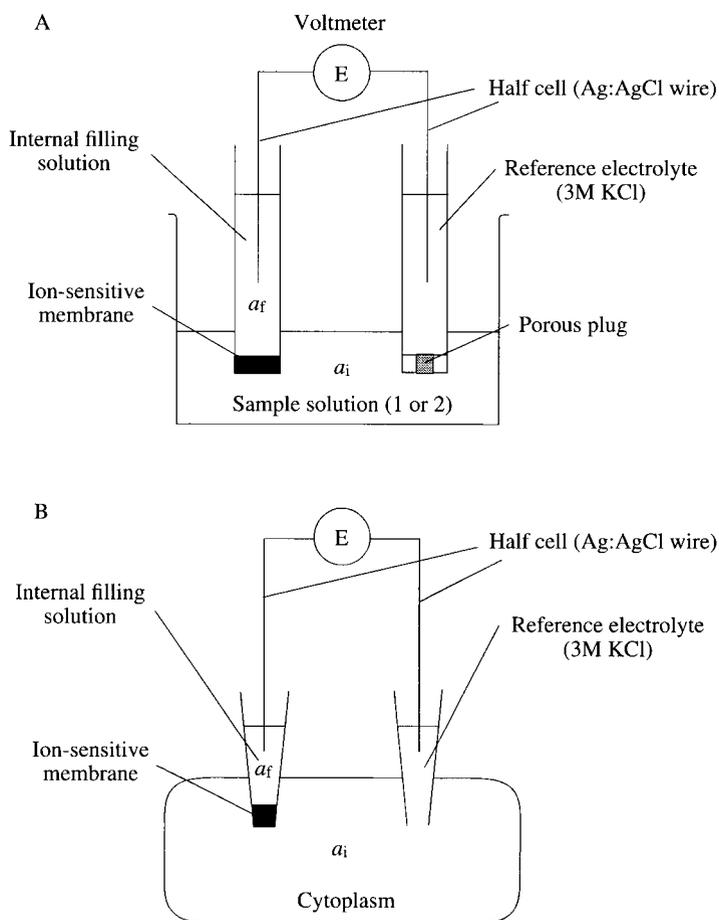
Fig. 2. Experimental set-up for ion-sensitive electrodes. The potential difference  $E$ , which exists across a selectively permeable membrane is measured by a voltmeter.  $a_f$  and  $a_i$  denote the activity of the permeant ion in the filling solution and in the sample solution respectively. For details, see text.
