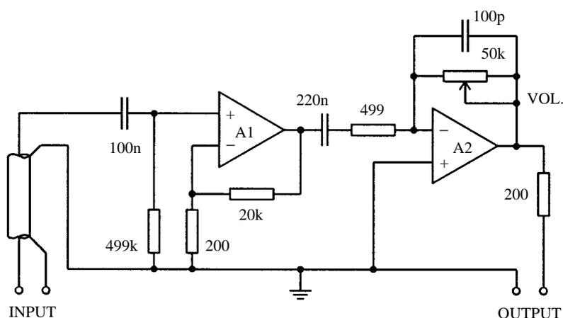
Fig. 8. Circuit diagram of a simple audio amplifier for headphones and a piezocrystal detector used in dry-bevelling of micropipettes. A1 is a low-noise op. amp. (e.g. LM 607), A2 is a general purpose op. amp. (e.g. LF 356). The circuit may be powered by two 9 V batteries or from a conventional  $\pm 15$  VDC source.
