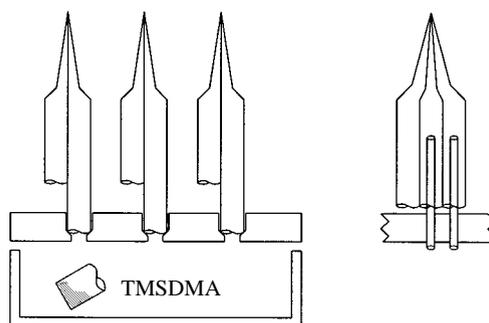
Fig. 6. Holder that allows selective silanization of individual barrels of double or triple-barrelled micropipettes. For details, see text.
