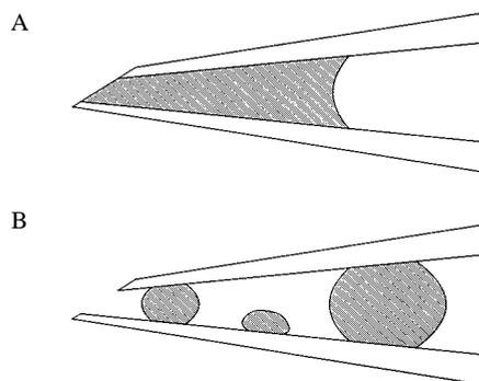
Fig. 4. (A) In a properly silanized micropipette, the liquid membrane solution forms a uniform column with a concave interface against the aqueous filling solution. (B) In a poorly silanized micropipette, the organic membrane solution is easily replaced by water at the hydrophilic glass surface which results in convex interfaces and, often, breaking of the membrane column.
