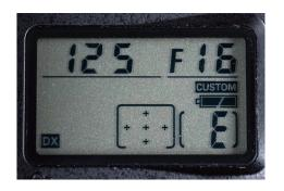
This camera is set at 1/125 second shutter speed and an F stop or aperture setting of F16.
