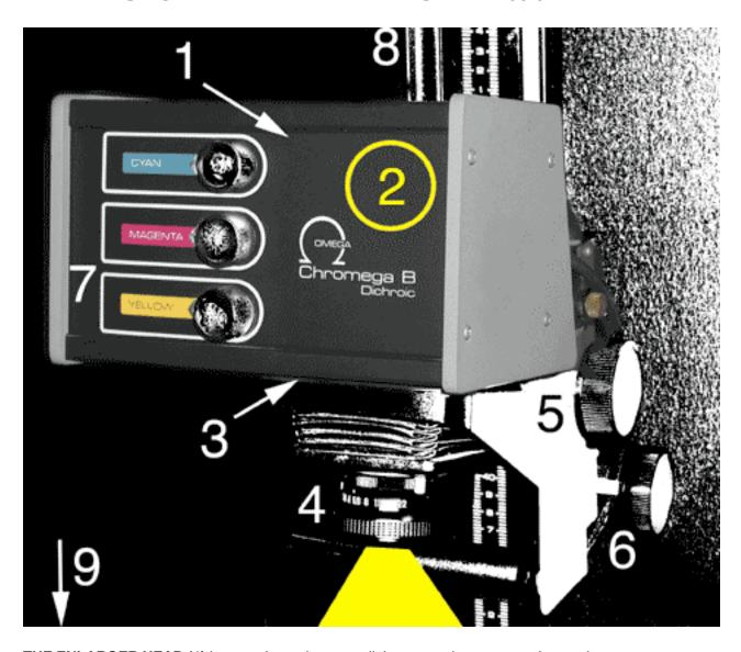
**THE ENLARGER HEAD (1)** houses the major parts--light source, lenses, negative carriers. Raising it up or down determines the size of the image.
