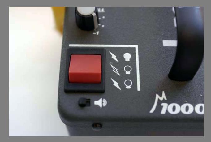
The on/off sound switch is positioned below the power switch. The beep indicates when the capacitors have a full charge. Always wait for the beep before making another exposure to avoid "racing the pack" and damaging the unit.
