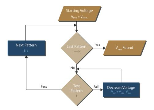
Fig. 1: Typical V<sub>min</sub> Search
