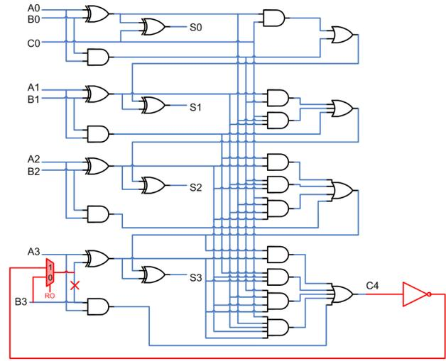
Fig. 1. The gate-level schematic of the 4-bit carry look-ahead adder and one constructed RO
