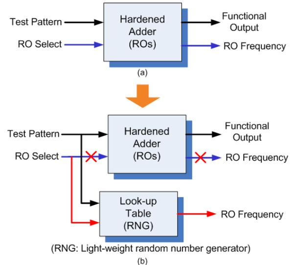
Fig. 2. The working procedure of (a) the original hardened adder, and (b) the Trojan-infested adder with a muted hardening scheme
